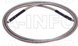
1.85M-1.85F-B010S-2000 Flexible Cable Assembly 2000mm DC- 67GHz 1.85mm Male to 1.85mm Female
